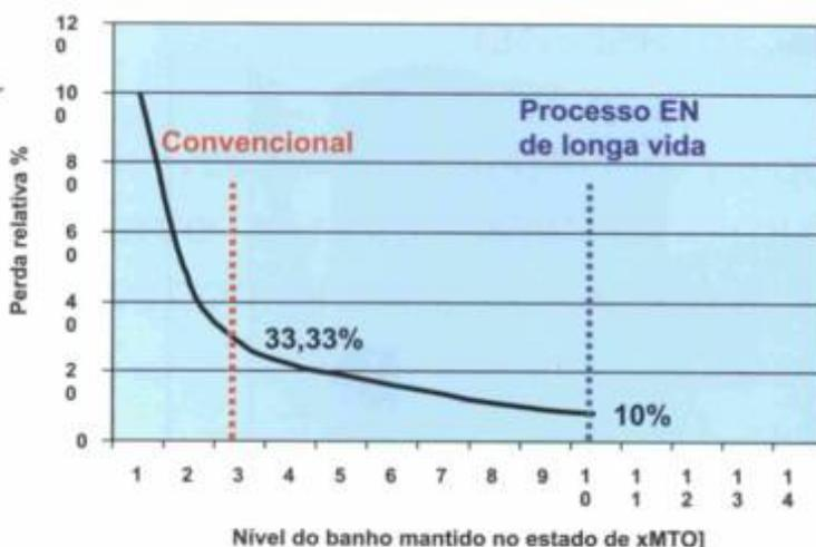
Figura 4 - Perda de material com "bleed and feed"
