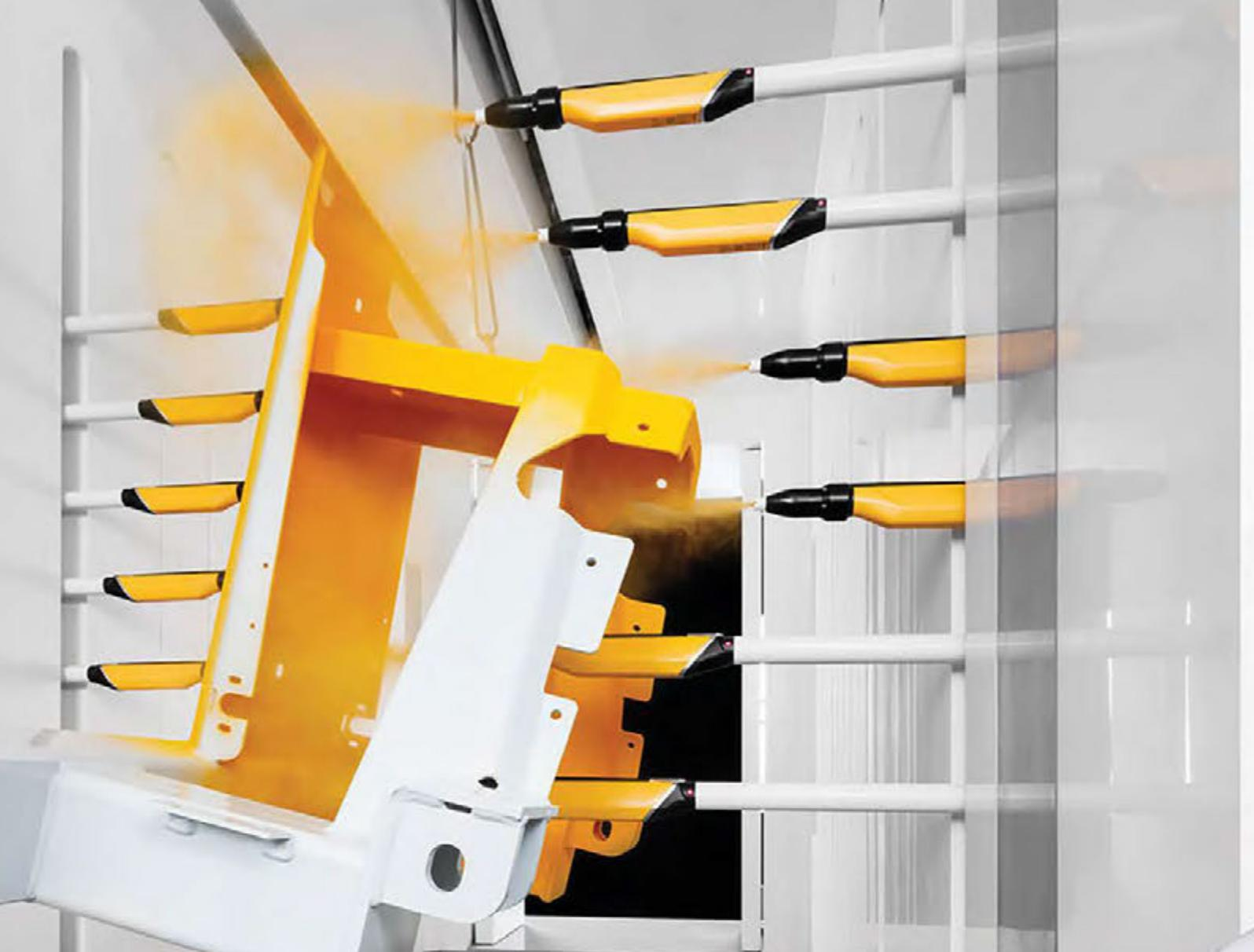
A close-up photograph of an industrial spray painting process. A yellow mechanical part is being painted by several spray guns. The spray guns are yellow and black, and they are spraying a fine mist of paint onto the part. The background is a white industrial structure.
